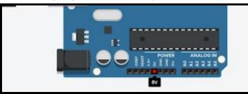
b. Hardware: plug a jumper wire into the 5V pin on the arduino and into the + power column on the breadboard.
